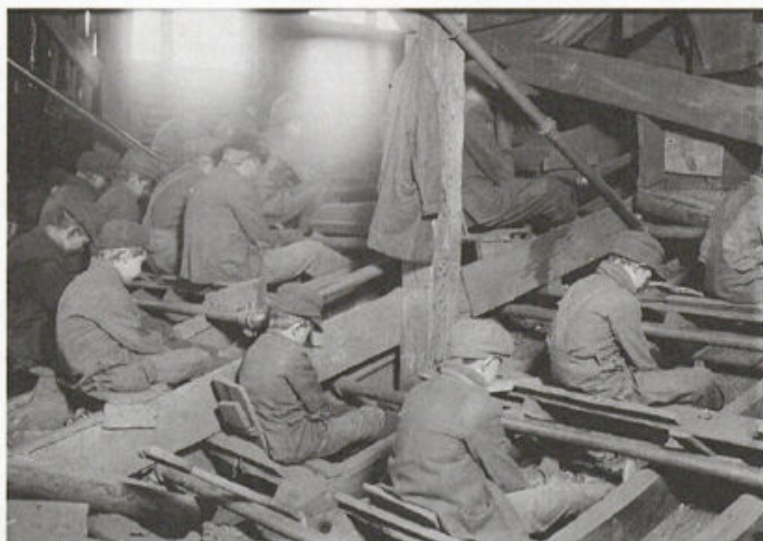
Breaker boys sort coal in an anthracite coal breaker near South Pittston, Pennsylvania, in 1911. Photo: Lewis Hine for the National Child Labor Committee.
